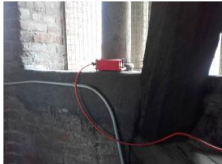
Figure 9: View of the seismometers and recorders to be installed in the Milan Cathedral [12, 13-14].
