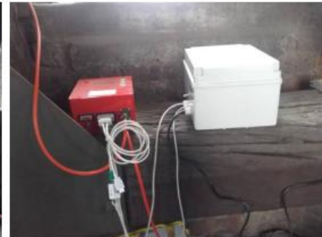
Figure 9: View of the seismometers and recorders to be installed in the Milan Cathedral [12, 13-14].
