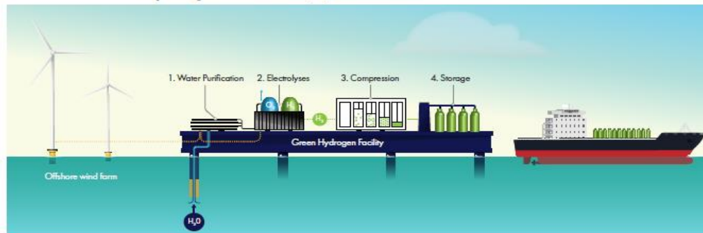
Offshore wind to hydrogen solution 1(b)
