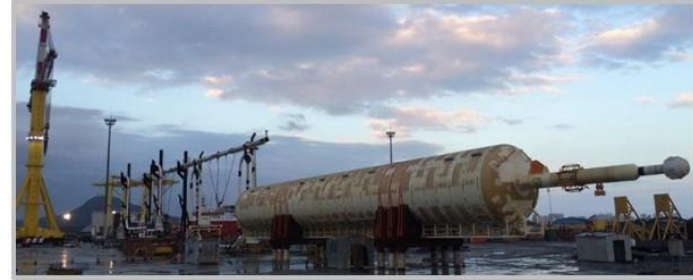
Load-Out Bouyancy Tank
