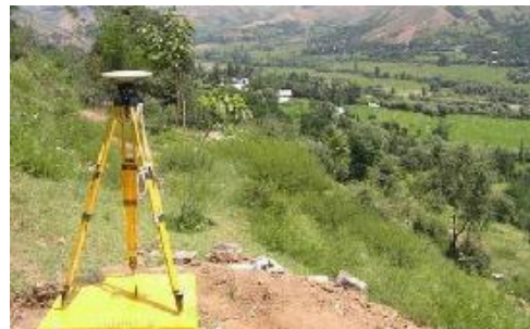
GPS-measurement for a tunnel network (Pir Panjal, India)
