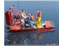
Fig3-Biological larvicide application with aerobote
