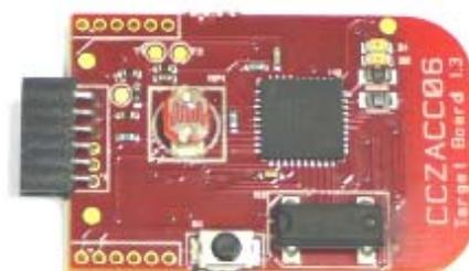
Figura 9: eZ430-RF2480 Target Board
